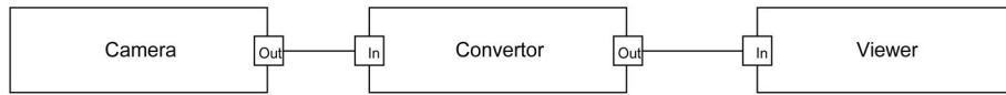
Fig. 8. A trivial scenario in which the atomic replacement of components could be required.
